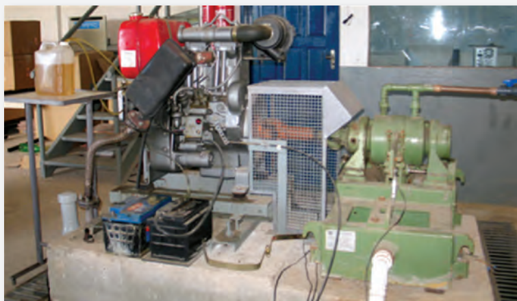
Figure 3. Diesel engine mounted on a dynamometer steady.
